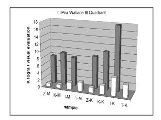
Figure 3. The results of rub-off resistance test measured by both methods; Pira Wallace and Quadrant.
