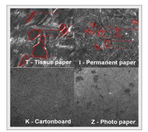
Figure 1. Surface topography, CLSM method
