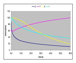
Figure 2. The results of PDA penetration test
